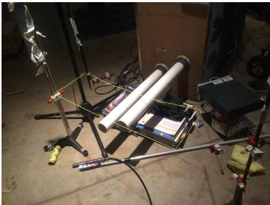
Figure 5.15 Settings for sound pressure measurement in working condition
