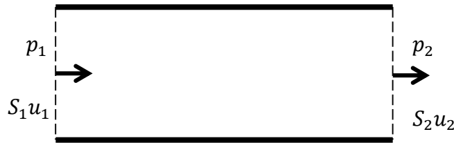
Figure 3.3 schematic of the variables and the sign convention for volume velocity
